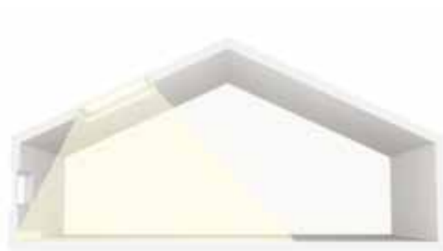
Adding a single roof window with a splayed internal lining can bring useful extra light into a room.
